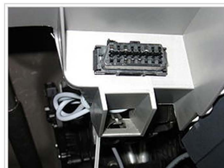
Female OBD-II connector fitted to a vehicle
